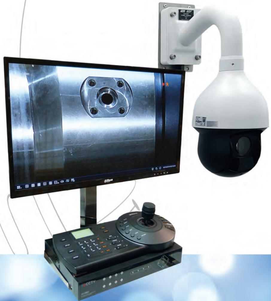
*Eztek's Safeye camera systems provide interference free imaging, increasing safety in workshops and on oil rigs.*
